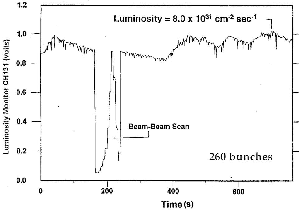
$$\mathcal{L}_{\text{measured}} = 8.0 \times 10^{31} \text{ cm}^{-2} \text{ sec}^{-1} \quad I^+ = 260 \text{ mA} \quad \Sigma_y = 14 \text{ } \mu\text{m} \quad \tau_+ = 24 \text{ min}$$
